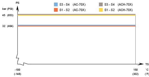
**AC70X / ACH70X – CRN approval pressure/temperature graph\***
