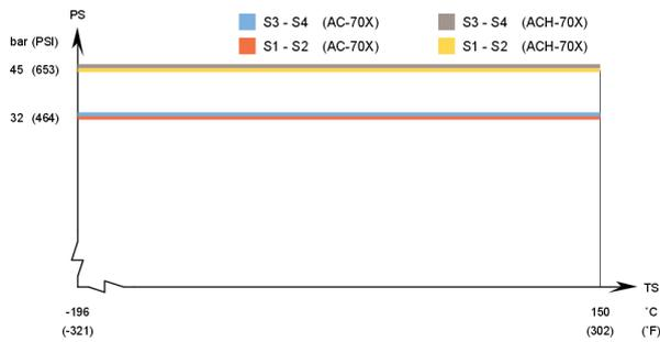
**AC70X / ACH70X – UL approval pressure/temperature graph\***
